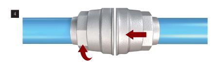
4. Only for tube diameters D50 and D63mm. To facilitate installation, fittings are supplied with unscrewed nuts. Once the tube is inserted into the fitting, tighten the nuts to the torque specified below.
